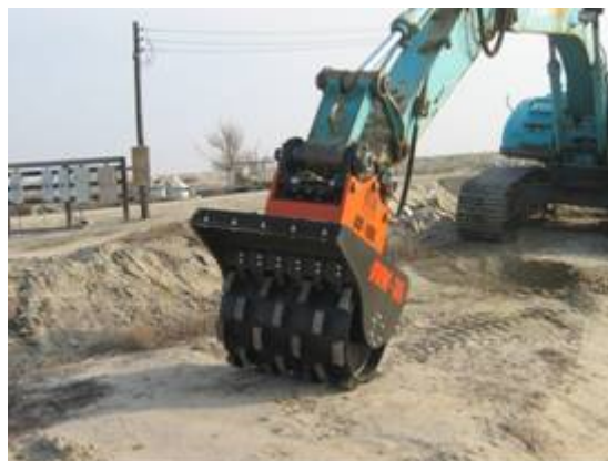
Figure 5. MBW 36” vibratory roller attached to the end of an excavator arm.
